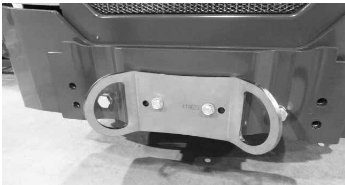
Tie down bracket A418623 installed at the rear bumper or counterweight
